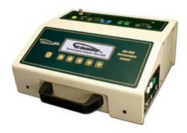
The ESU-2300 Analyser is for users who prefer a conventional instrument with internal, selectable test loads. Utilising the same Patent-Pending DFATM Technology as our new ESU-2050, and ESU-2400, the ESU-2300 uses industry standard current sensing technology rather than relying on less accurate voltage measurement techniques offered by some competitive products.
